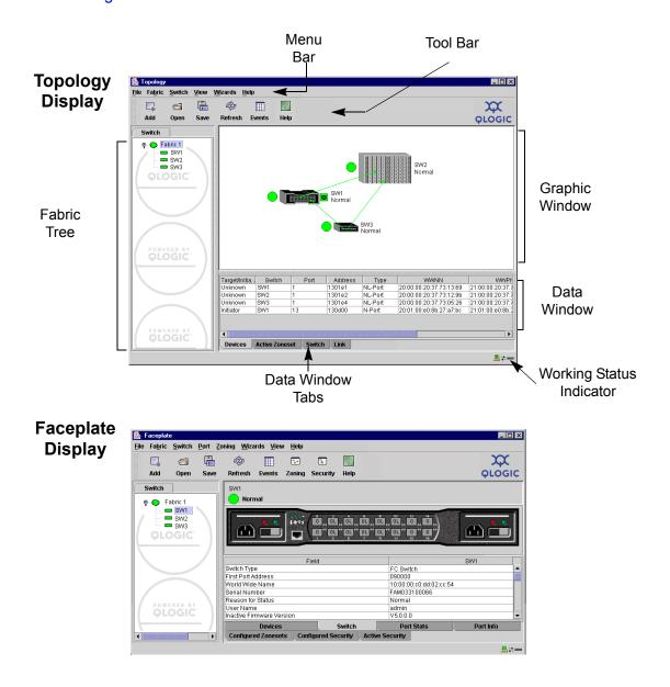
Figure 2-6. SANsurfer Switch Manager Display Elements
